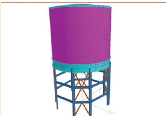
1973 m 3 Silo for Cement Industry in India
